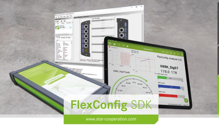
FlexConfig SDK is a .NET lib for the easy access of automotive bus systems in your own windows applications. The library supports a wide range of automotive network description formats like FIBEX, AUTOSAR (.arxml) or CANdb.
